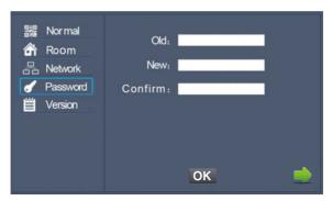
You can set the new system password with 1-16 digits (the default password is 123456). System password is used for system settings.
