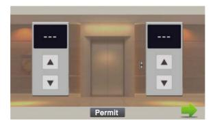
Click or icon to control the up and down of the elevator. Click "Permit" icon to permit access to the floor where the indoor monitor locates.
