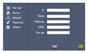
IP: the system will automatically display IP address of the indoor monitor. IP address is unique.
