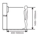
【 Suggestion】: During the installation, the camera should be 1450∼1550mm above the ground. The camera tether for photographing human face should be the top priority.
