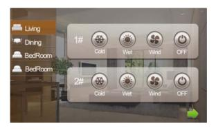
Set the air-condition switch of corresponding room. Click "OFF" icon to turn air-conditioner on/off; click "Cold" icon to cool; click "Wet" icon to dehumidify; click "Wind" icon to ventilate.
