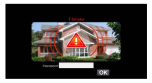
You can see the No. and sensor type in red color showed at the top of interface. Fox example, "2: Smoke" indicates that smoke sensor in zone 2 is triggered.
