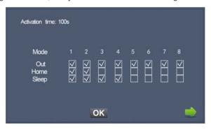
refers to Alarm ON, and refers to Alarm OFF. To set the sensor of alarm stations, you can click the corresponding station with license icon. Click activation time to choose the corresponding time. The options of activation time include NONE, 30s, 40s, 60s, 100s and 300s.
