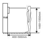
【 Suggestion】: During the installation, the camera should be 1450∼1550mm above the ground. The camera tether for photographing human face should be the top priority.
