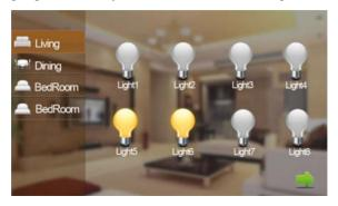
Set the light of corresponding room, such as Master Bedroom, Secondary Bedroom, Living Room and Dining Room (see the room setting for details). 8 lights can be set in every room at most. Clicking the corresponding light icon, you can turn the light ON/OFF.
