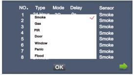
When alarm sensor is triggered, the indoor monitor will make a loud alarm sound, and the system will enter into the following interface as well as send alarm message to management center (if management center is available in your system):
